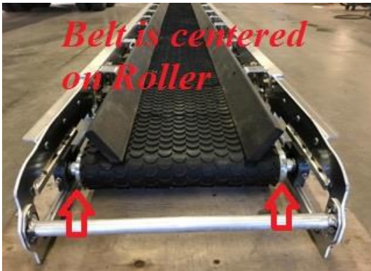
This belt is tracking correctly.
