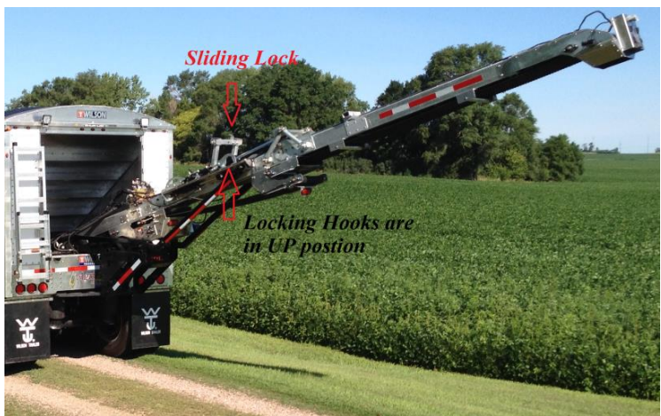
Conveyor is Raised all the way UP, when Folding & Unfolding.
