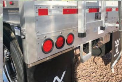
Wilson's deeper front/rear channels add strength to the trailer's design.
