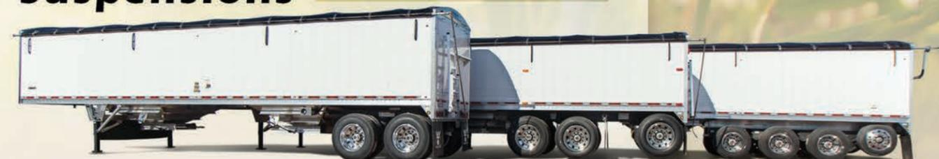
Wilson offers a variety of suspension configurations; tandem, spread axle, tri-axle and quad axle. Talk with your Authorized Wilson Sales Representative about which suspension will work best for you.
