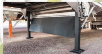
Full-width belting between landing gear legs
