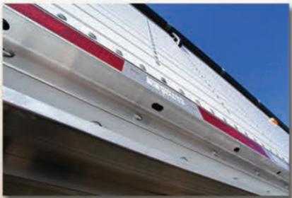
Side vent ports, positioned between each set of side posts, allow the sides to breathe, extend the life of the side wall, and also serve as a useful inspection source.
