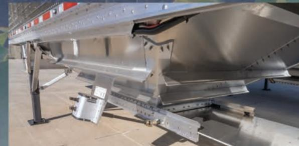
RRP traps with 2-speed gear boxes are used for larger sized doors, metering fertilizer and seed, and hauling sand and aggregate.
