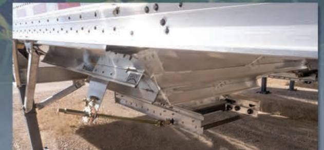
RRP traps with direct drive are used for smaller doors and ag commodities. (Shown with standard steel door. Optional aluminum & stainless steel doors are available)
