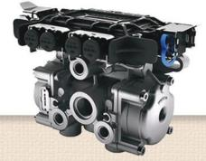
2-sensor/1-modulator (2S/1M) is the mandatory minimum for ABS valves on all trailers. **Enhance the ABS anti-skid performance and directional stability with more sensors** such as a 4S/2M configuration.
