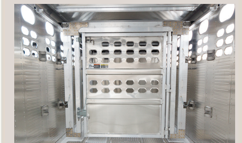
Style-O Improved Roller Gate with Multiple Settings
