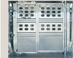
Style-C – Optional Gate with Inner Slide.
