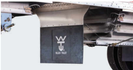
48" wide, one-piece mud flap in front of rear trap mounted to stiffener
