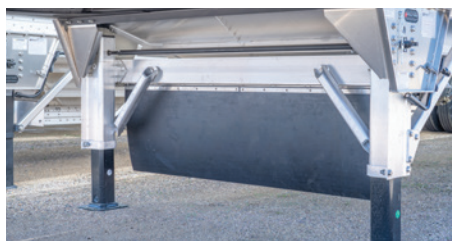
Full-width belting between landing gear legs
