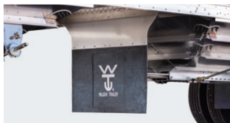
48" wide, one-piece mud flap in front of rear trap mounted to stiffener
