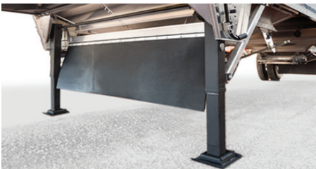
Full-width belting between landing gear legs
