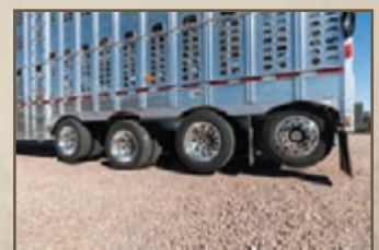
Quad axle with rear lift/steer axle and load-sensed auto drop for axles 1 & 3
