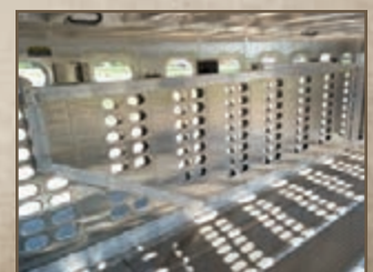
Bull Bar Punched to Match Side
