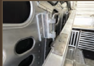
Spring Loaded Auto Latch for Fold to Wall Ramp
