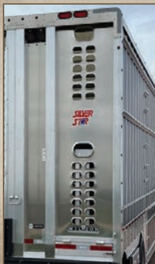
Rear Pan Punched to Match Side
