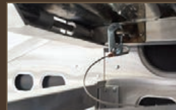
Cable Hold-back Keeps No-Step Ramp in Place During Transport. (Standard on Drop Center Trailers, Optional on Straight Floors)
