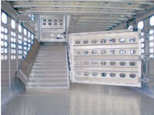
Folding removable bullbar with pull-out ramp in loading position.
