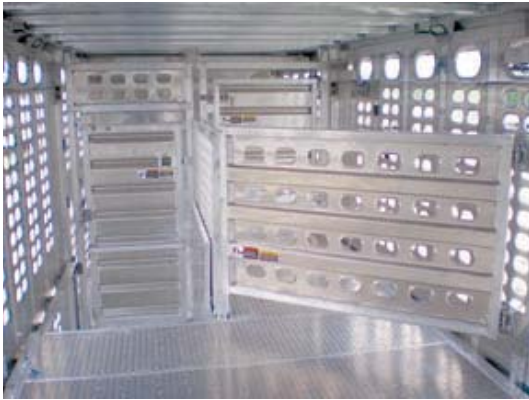
Drop ramp option with funnel/door brace in loading position.
