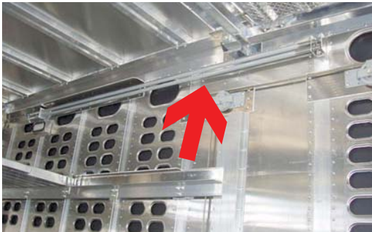
Side brace rods must be in place under the deck to prevent trailer side deflection when the trailer is being used to haul livestock.
