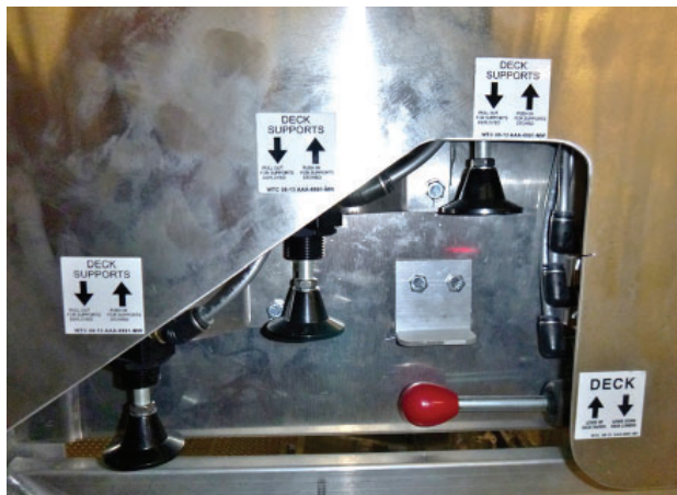
Control Station Function Labels
