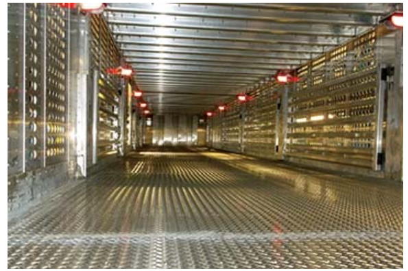
Air Operated Deck Support Deployed
