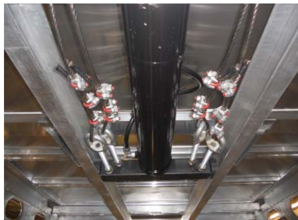
Hydraulic Cylinder with Rope Ends Connected to Wheeled Trolley
