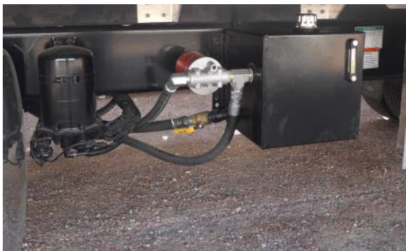
Hydraulic Power Take Off Reservoir Truck Mounted
