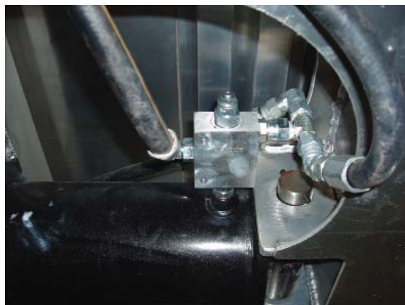
Load Holding Hydraulic Valve Mounted to Hydraulic Cylinder
