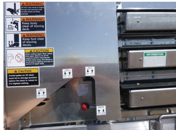
Warning and Caution Labels at Control Station
