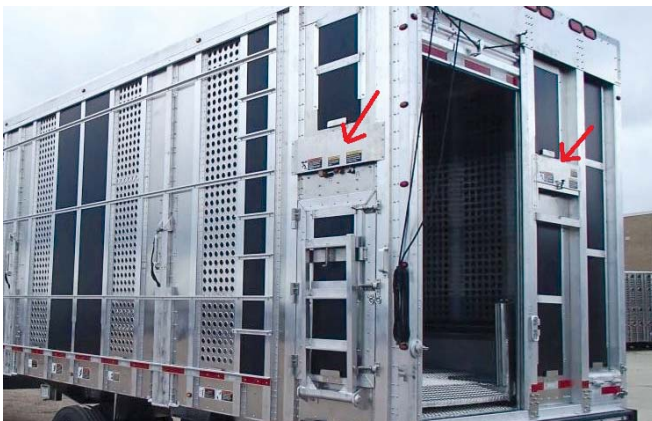
Air Controls for Deck Support Rear Station
