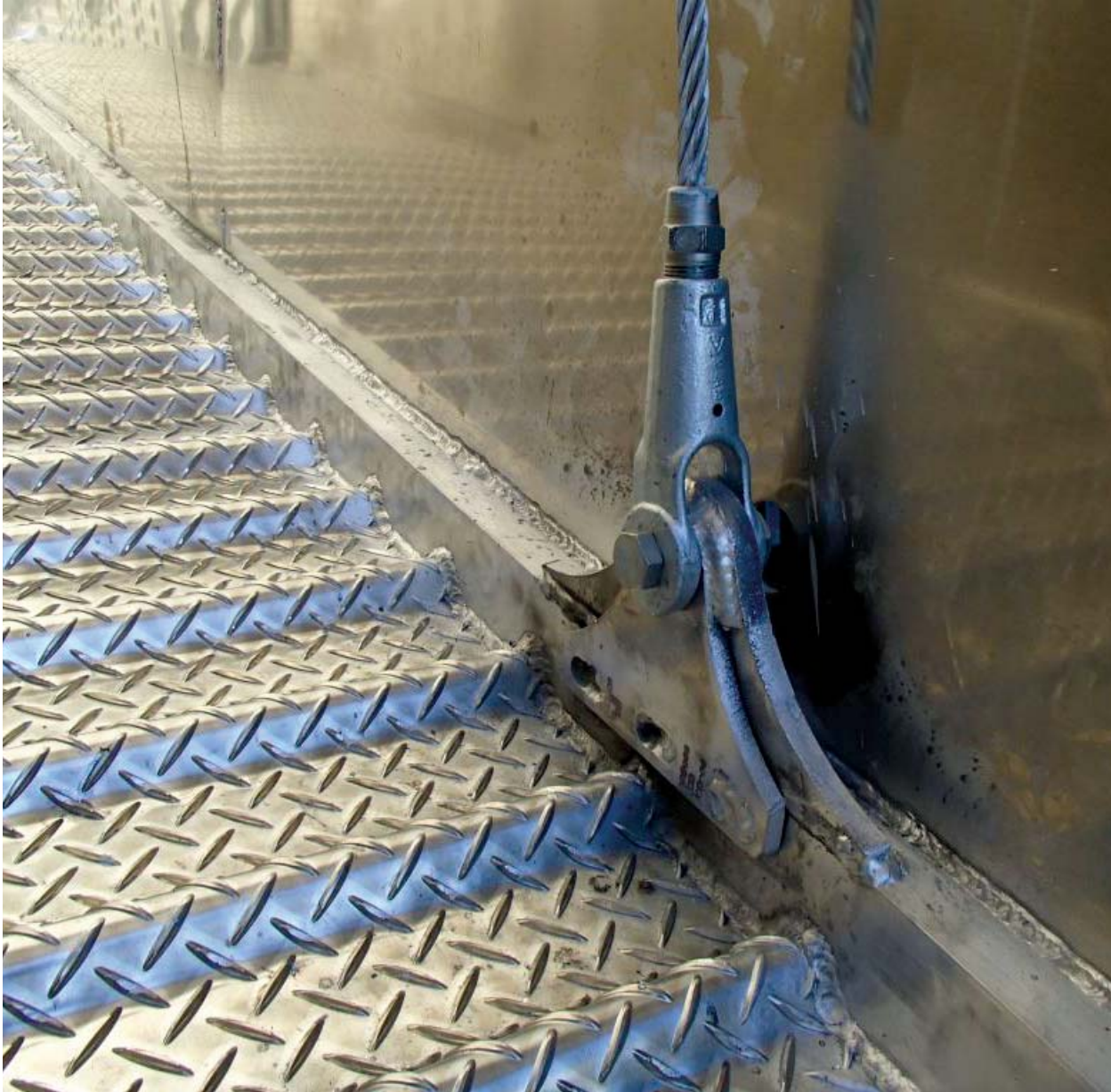
Wire Rope Connections to Ramp
